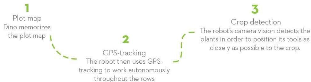
GPS-guidance is paired with camera vision in order for Dino to be operational in a maximum of configurations while keeping its precision range.
